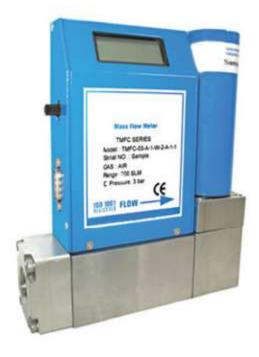
Bass Instruments, TMFC series Thermal Mass Controller is an instrument designed to measure dry gas and control flow rate without affecting pressure and temperature. You can adjust the flow control with manual set button or 0-5 VDC input signal. AISI316 body up to 35 bar can be used.
